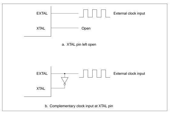
Figure 19.5 External Clock Input (Examples)
