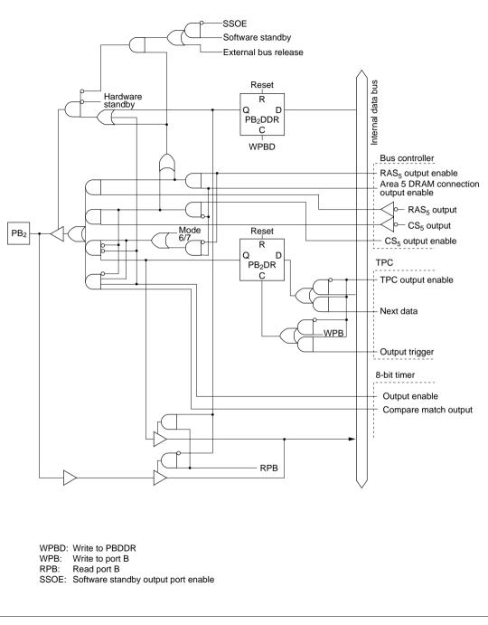
Figure C.11 (c) Port B Block Diagram (Pin PB<sub>2</sub>)
