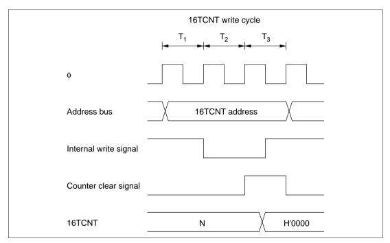
Figure 9.37 Contention between 16TCNT Write and Clear
