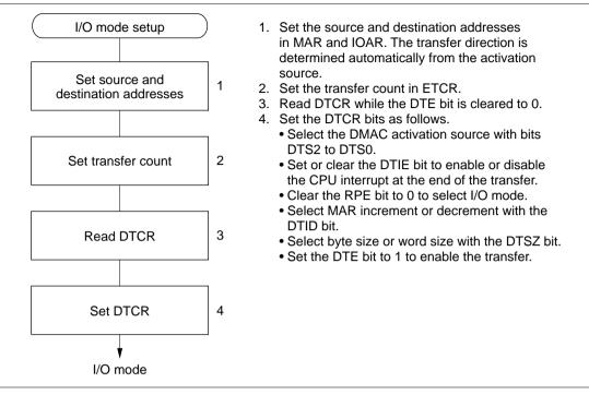
Figure 7.3 I/O Mode Setup Procedure (Example)
