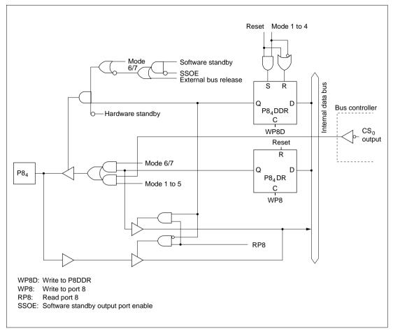
Figure C.8 (e) Port 8 Block Diagram (Pin P8<sub>4</sub>)
