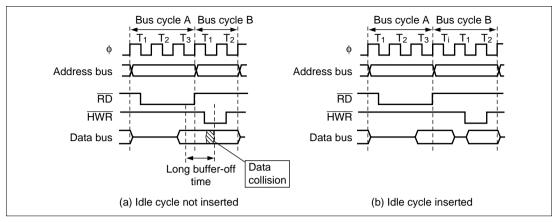
Figure 6.44 Example of Idle Cycle Operation (2) (ICIS0 = 1)
