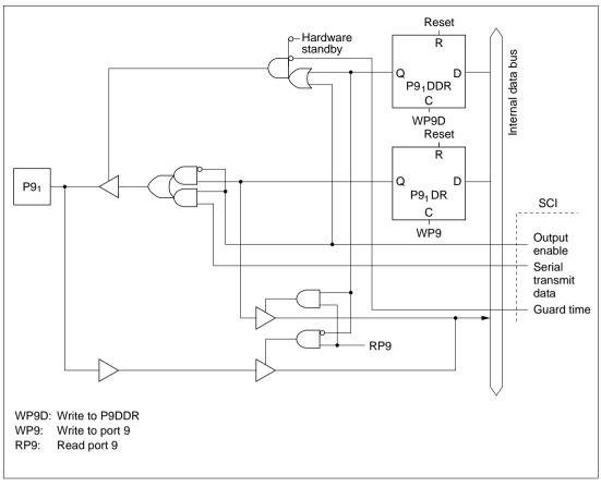
Figure C.9 (b) Port 9 Block Diagram (Pin P9<sub>1</sub>)
