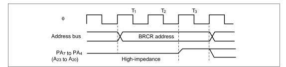
Figure 6.51 BRCR Write Timing
