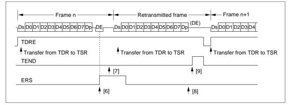
Figure 14.13 Retransmission in SCI Transmit Mode
