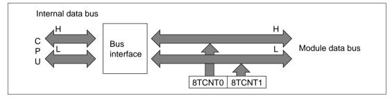
Figure 10.3 8TCNT Access Operation (CPU Reads 8TCNT, Word)
