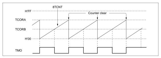
Figure 10.17 Example of Pulse Output
