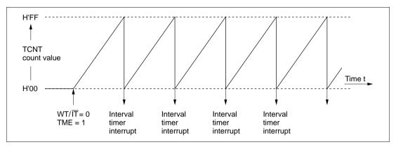
Figure 12.5 Interval Timer Operation
