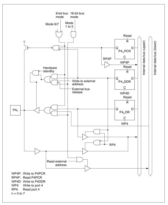
Figure C.4 Port 4 Block Diagram
