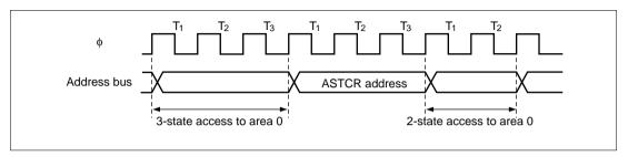
Figure 6.49 ASTCR Write Timing
