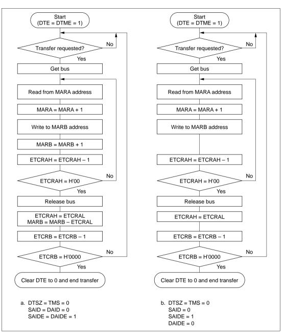
Figure 7.11 Block Transfer Mode Flowcharts (Examples)
