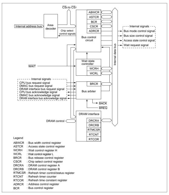
Figure 6.1 Block Diagram of Bus Controller
