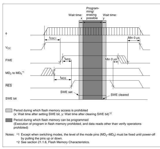
Figure 18.16 Power-On/Off Timing (Boot Mode)
