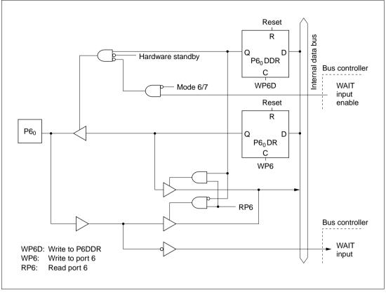
Figure C.6 (a) Port 6 Block Diagram (Pin P6<sub>0</sub>)
