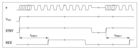
Figure 21.4 Oscillator Settling Timing
