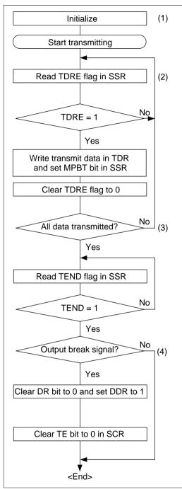
SCI initialization: the transmit data output function of the TxD pin is selected automatically.
