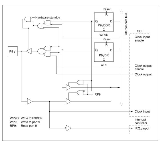
Figure C.9 (e) Port 9 Block Diagram (Pin P9<sub>4</sub>)
