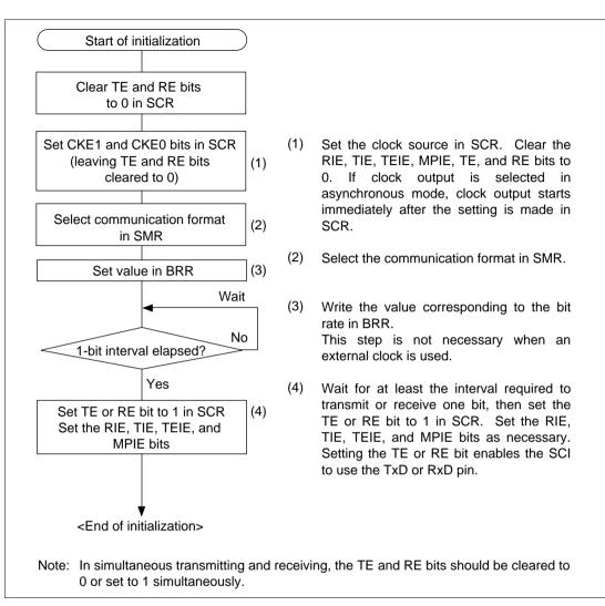
Figure 13.4 Sample Flowchart for SCI Initialization
