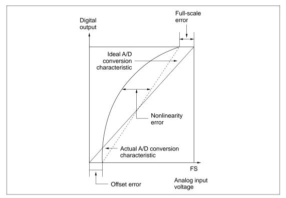
Figure 15.10 A/D Converter Accuracy Definitions (2)
