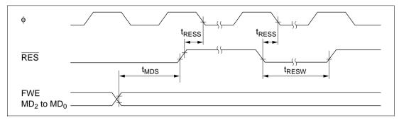
Figure 21.5 Reset Input Timing
