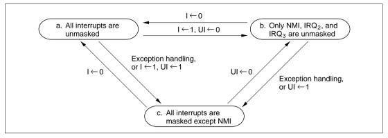
Figure 5.5 Interrupt Masking State Transitions (Example)
