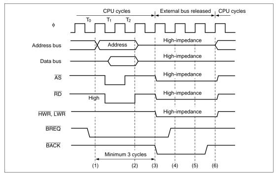
Figure 6.48 Example of External Bus Master Operation
