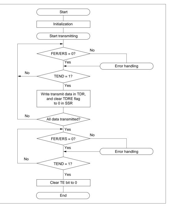
Figure 14.5 Sample Transmission Processing Flowchart
