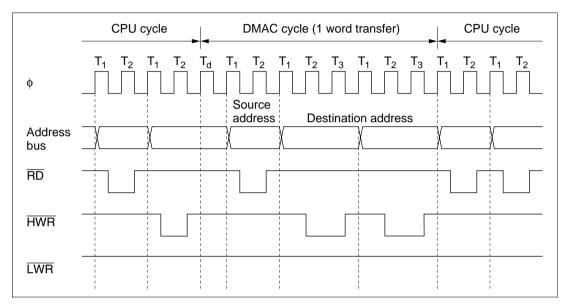
Figure 7.13 DMA Transfer Bus Timing (Example)
