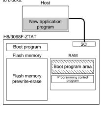
Programming control program transfer When boot mode is entered, the boot program in the H8/3068F-ZTAT (originally incorporated in the chip) is started and the programming control program in the host is transferred to RAM via SCI communication. The boot program required for flash memory erasing is automatically transferred to the RAM boot program area.
