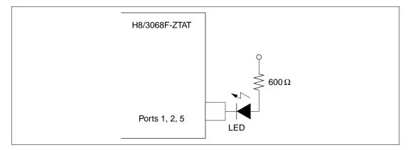
Figure 21.2 Sample LED Circuit
