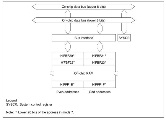
Figure 17.1 RAM Block Diagram
