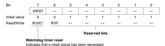
Notes: RSTCSR is write-protected by a password. For details see section 12.2.4, Notes on Register Access.
