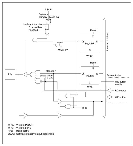
Figure C.6 (e) Port 6 Block Diagram (Pin P6<sub>4</sub>)
