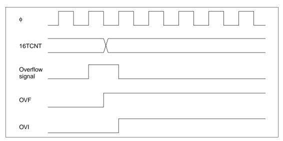
Figure 9.35 Timing of Setting of OVF
