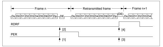
Figure 14.12 Retransmission in SCI Receive Mode
