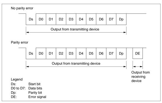
Figure 14.3 Smart Card Interface Data Format
