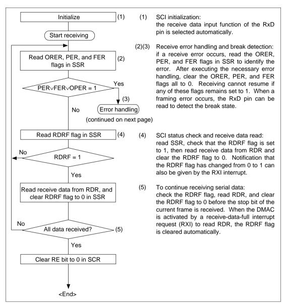
Figure 13.7 Sample Flowchart for Receiving Serial Data (1)
