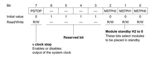
MSTCRH is initialized to H'78 by a reset and in hardware standby mode. It is not initialized in software standby mode.
