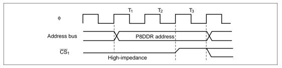
Figure 6.50 DDR Write Timing
