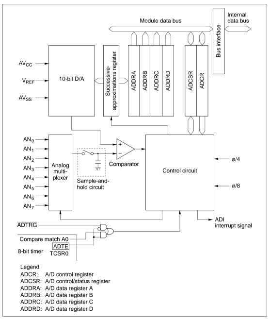
Figure 15.1 A/D Converter Block Diagram
