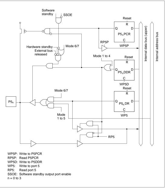
Figure C.5 Port 5 Block Diagram
