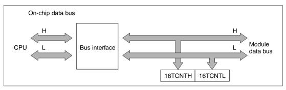
Figure 9.4 16TCNT Access Operation [CPU  $\rightarrow$  16TCNT (Word)]
