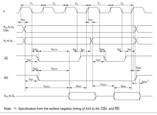
Figure 21.11 Burst ROM Access Timing: Two-State Access
