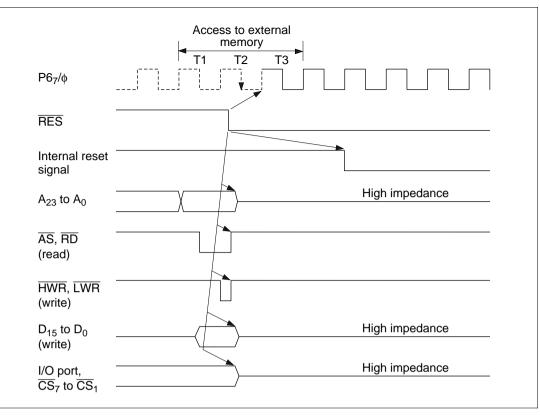
Figure D.3 Reset during Memory Access (Mode 5)
