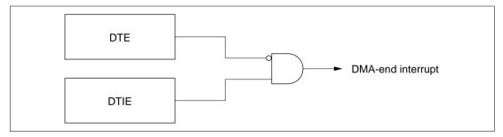
Figure 7.25 DMA-End Interrupt Logic
