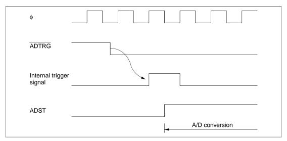
Figure 15.6 External Trigger Input Timing
