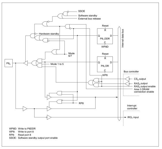
Figure C.8 (b) Port 8 Block Diagram (Pin P8<sub>1</sub>)
