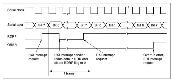
Figure 13.19 Example of SCI Receive Operation
