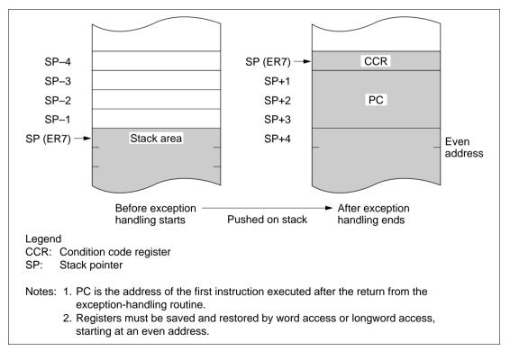
Figure 2.14 shows the stack after the exception-handling sequence.
