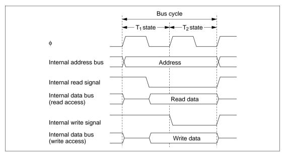
Figure 2.15 On-Chip Memory Access Cycle
