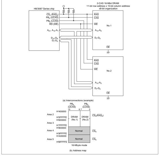
Figure 6.32 Interconnections and Address Map for 16-Mbit DRAMs with × 8-Bit Organization
