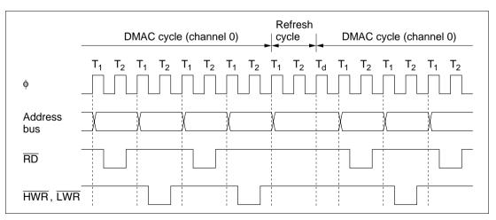
Figure 7.20 Bus Timing of DRAM Interface, and DMAC
