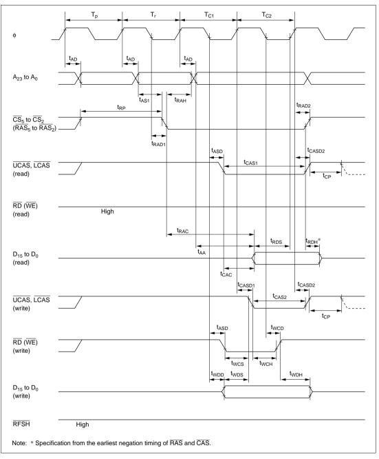
Figure 21.14 DRAM Bus Timing (Read/Write)
