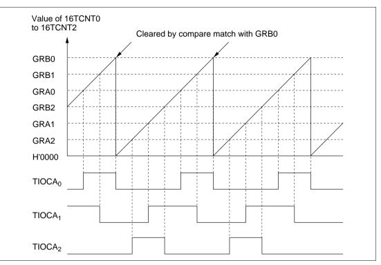
Figure 9.25 Synchronization (Example)
