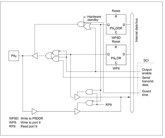
Figure C.9 (a) Port 9 Block Diagram (Pin P9<sub>0</sub>)
