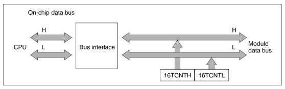
Figure 9.5 Access to Timer Counter (CPU Reads 16TCNT, Word)
