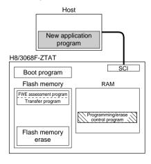
Programming/erase control program transfer When user program mode is entered, user software recognizes this fact, executes the transfer program in the flash memory, and transfers the programming/erase control program to RAM.
