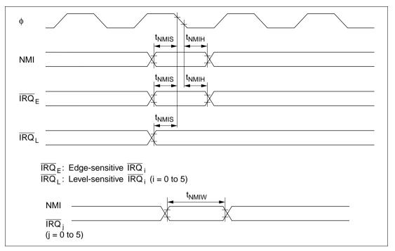
Figure 21.7 Interrupt Input Timing
