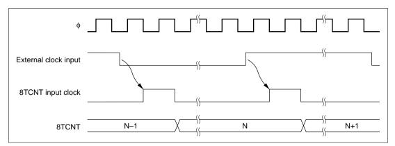
Figure 10.9 Count Timing for External Clock Input (Both-Edge Detection)
