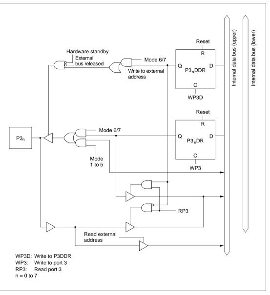
Figure C.3 Port 3 Block Diagram
