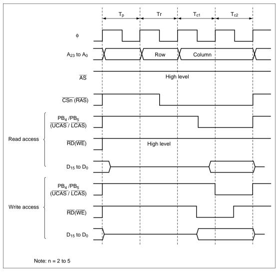
Figure 6.18 Basic Access Timing (CSEL = 0 in DRCRB)
