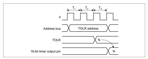
Figure 9.32 Timing for Setting 16-Bit Timer Output Level by Writing to TOLR
