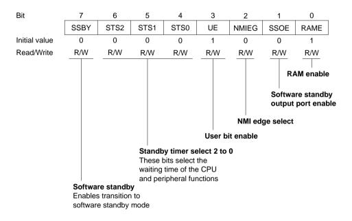
SYSCR is an 8-bit readable/writable register. Bit 7 (SSBY), bits 6 to 4 (STS2 to STS0), and bit 1 (SSOE) control the power-down state. For information on the other SYSCR bits, see section 3.3, System Control Register (SYSCR).
