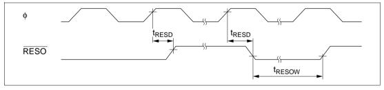
Figure 21.6 Reset Output Timing\*
