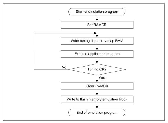
Figure 18.13 Flowchart of Flash Memory Emulation in RAM
