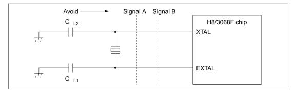
Figure 19.4 Oscillator Circuit Block Board Design Precautions
