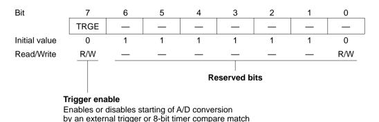
ADCR is an 8-bit readable/writable register that enables or disables starting of A/D conversion by external trigger input or an 8-bit timer compare match signal. ADCR is initialized to H'7F by a reset and in standby mode.
