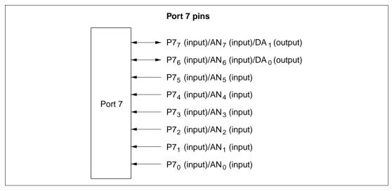
Figure 8.7 Port 7 Pin Configuration
