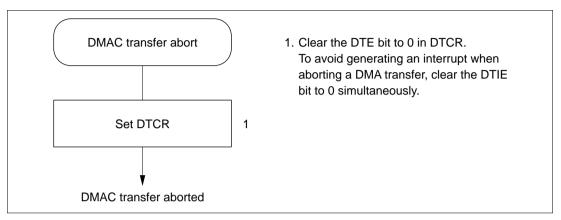
Figure 7.22 Procedure for Aborting a DMAC Transfer
