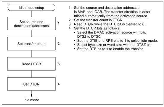
Figure 7.5 Idle Mode Setup Procedure (Example)
