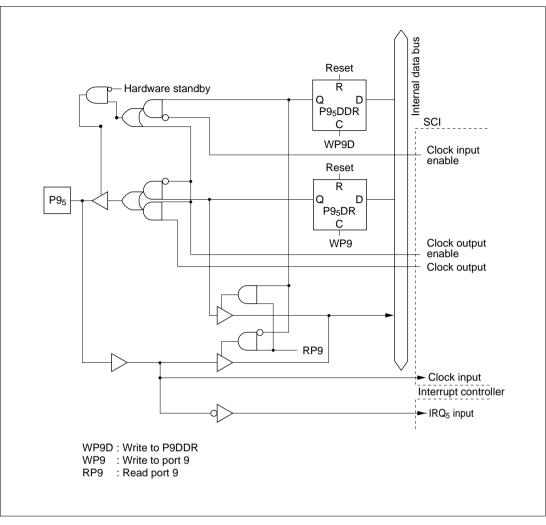
Figure C.9 (f) Port 9 Block Diagram (Pin P95)
