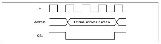
**Figure 6.4**  $\overline{\text{CS}}$ n Signal Output Timing (n = 0 to 7)
