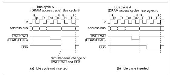
Figure 6.45 Example of Idle Cycle Operation (3) (HWR/LWR Used as UCAS/LCAS)
