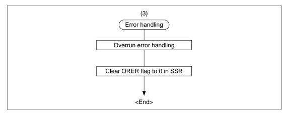
Figure 13.18 Sample Flowchart for Serial Receiving (2)
