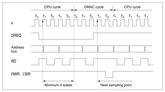
Figure 7.17 Timing of DMAC Activation by Low DREQ Level in Normal Mode
