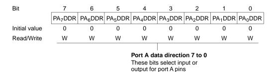
Port A is multiplexed with pins  $TP_7$  to  $TP_0$ . Bits corresponding to pins used for TPC output must be set to 1. For further information about PADDR, see section 8.11, Port A.
