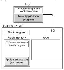
Flash memory initialization The programming/erase program in RAM is executed, and the flash memory is initialized (to H'FF). Erasing can be performed in block units, but not in byte units.
