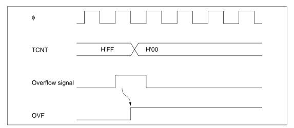
Figure 12.6 Timing of Setting of OVF
