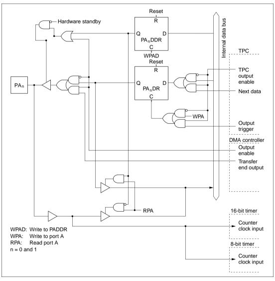
Figure C.10 (a) Port A Block Diagram (Pins PA<sub>0</sub>, PA<sub>1</sub>)
