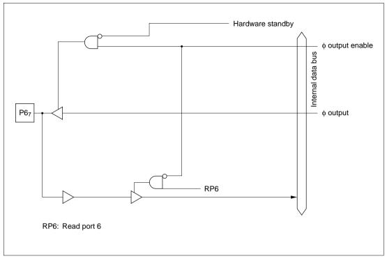
Figure C.6 (g) Port 6 Block Diagram (Pin P67)
