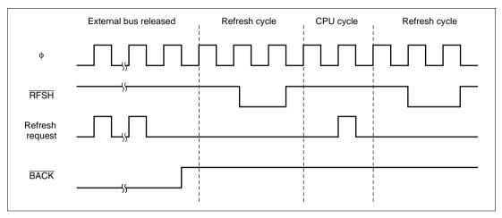
Figure 6.35 Bus-Released State and Refresh Cycles
