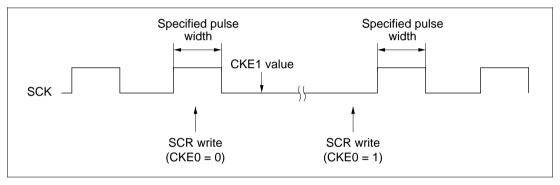
Figure 14.9 Timing for Fixing Cock Output
