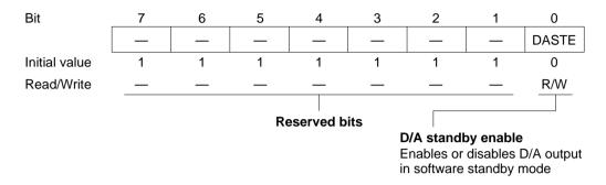
DASTCR is initialized to H'FE by a reset and in hardware standby mode. It is not initialized in software standby mode.
