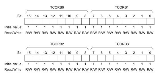
TCORB0 to TCORB3 are 8-bit readable/writable registers. The TCORB0 and TCORB1 pair, and the TCORB2 and TCORB3 pair, can each be accessed as a 16-bit register by word access.
