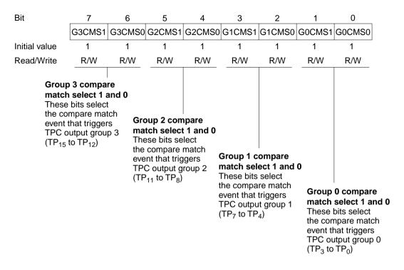
TPCR is initialized to H'FF by a reset and in hardware standby mode. It is not initialized in software standby mode.
