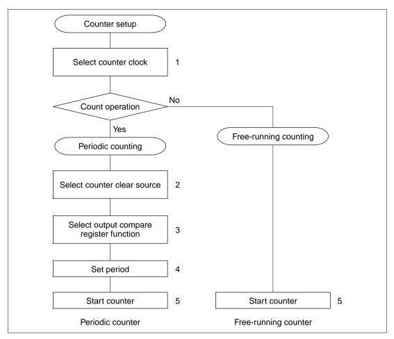
Figure 9.12 Counter Setup Procedure (Example)
