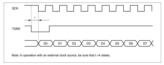
Figure 13.22 Example of Synchronous Transmission Using DMAC
