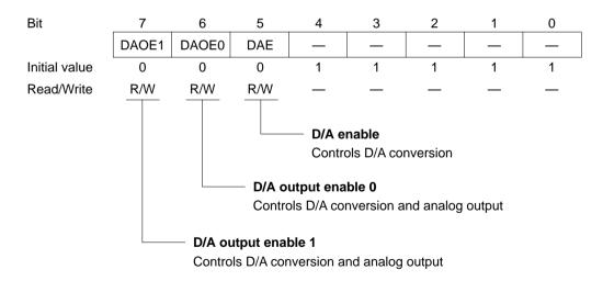
DACR is an 8-bit readable/writable register that controls the operation of the D/A converter. DACR is initialized to H'1F by a reset and in standby mode.
