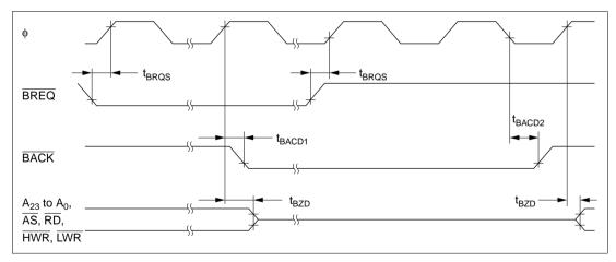
Figure 21.13 Bus-Release Mode Timing
