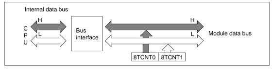
Figure 10.6 8TCNT0 Access Operation (CPU Reads 8TCNT0, Upper Byte)
