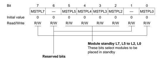
MSTCRL is initialized to H'00 by a reset and in hardware standby mode. It is not initialized in software standby mode.
