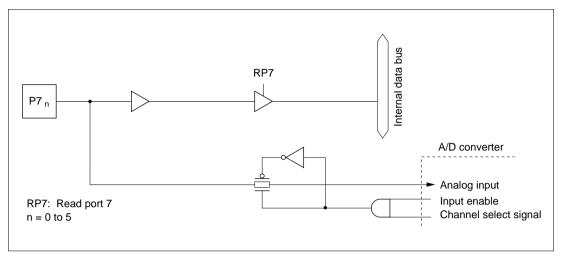
Figure C.7 (a) Port 7 Block Diagram (Pins P7<sub>0</sub> to P7<sub>5</sub>)
