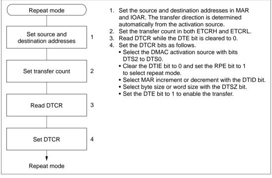
Figure 7.7 Repeat Mode Setup Procedure (Example)
