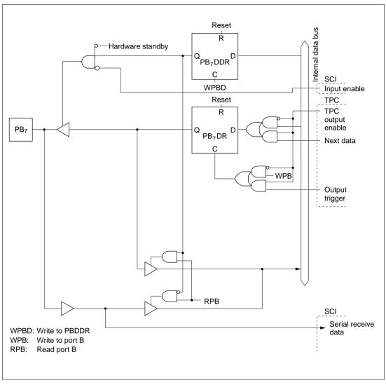
Figure C.11 (h) Port B Block Diagram (Pin PB<sub>7</sub>)
