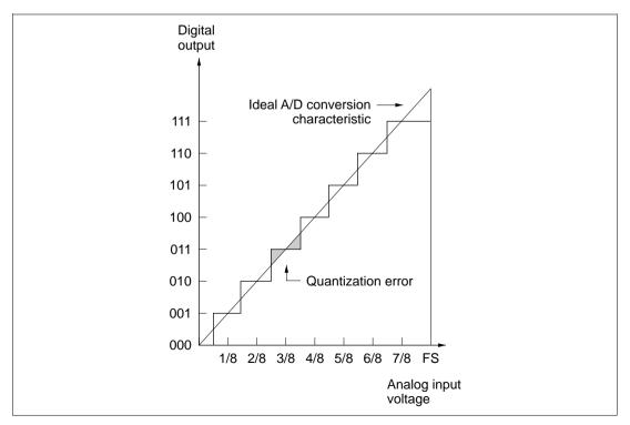
Figure 15.9 A/D Converter Accuracy Definitions (1)
