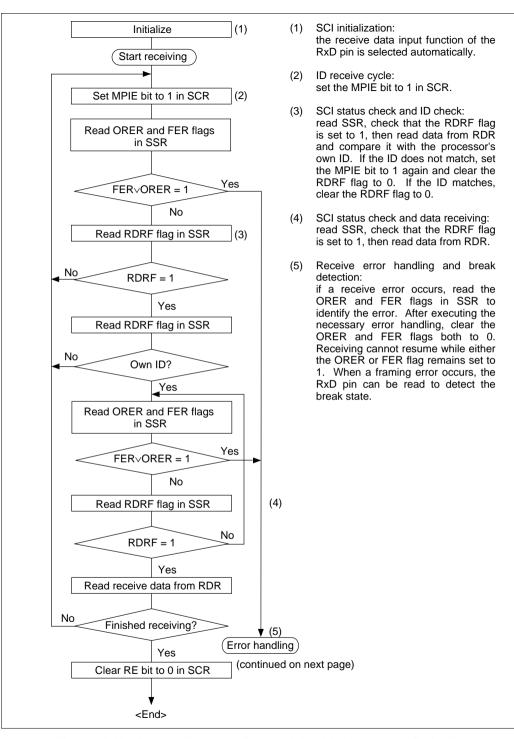
Figure 13.12 Sample Flowchart for Receiving Multiprocessor Serial Data (1)
