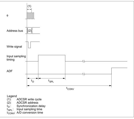
Figure 15.5 A/D Conversion Timing
