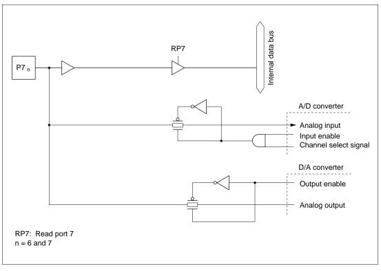
Figure C.7 (b) Port 7 Block Diagram (Pins P7<sub>6</sub> and P7<sub>7</sub>)
