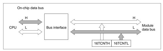
Figure 9.9 Access to Timer Counter L (CPU Reads 16TCNTL, Lower Byte)
