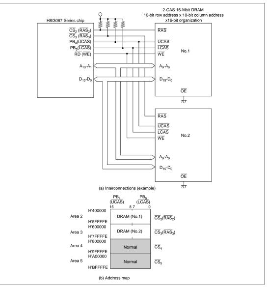
Figure 6.31 Interconnections and Address Map for 2-CAS 16-Mbit DRAMs with  $\times$  16-Bit Organization
