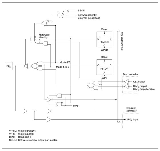
Figure C.8 (c) Port 8 Block Diagram (Pin P82)
