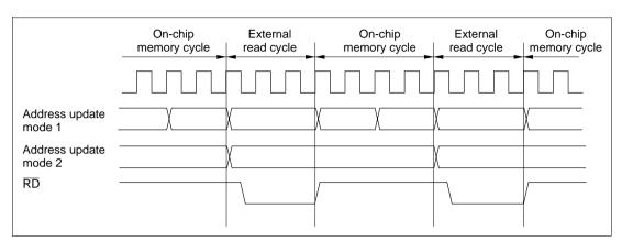
Figure 6.5 shows examples of address output in these two update modes.
