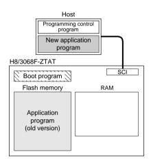
Flash memory initialization The erase program in the boot program area (in RAM) is executed, and the flash memory is initialized (to H'FF). In boot mode, total flash memory erasure is performed, without regard to blocks.
