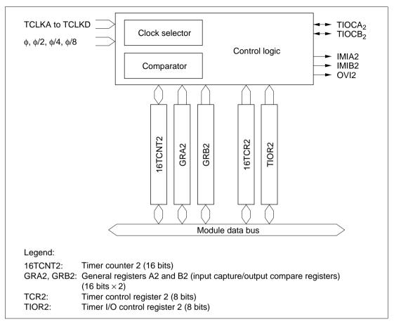
Figure 9.3 Block Diagram of Channel 2
