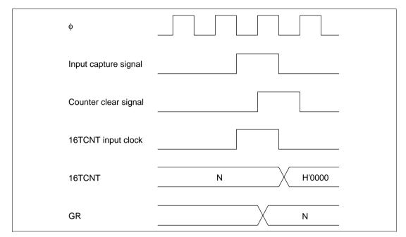
Figure 9.43 Contention between Counter Clearing by Input Capture and Counter Increment **Contention between General Register Write and Input Capture:** If an input capture signal occurs in the  $T_3$  state of a general register write cycle, input capture takes priority and the write to the general register is not performed. See figure 9.44.
