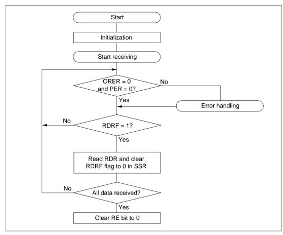
Figure 14.8 Sample Reception Processing Flowchart
