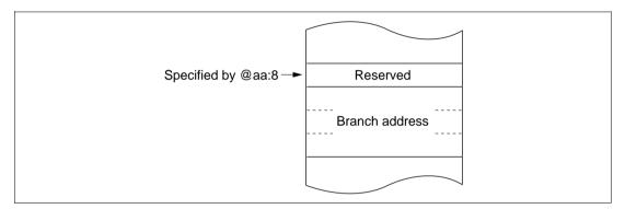
Figure 2.10 Memory-Indirect Branch Address Specification
