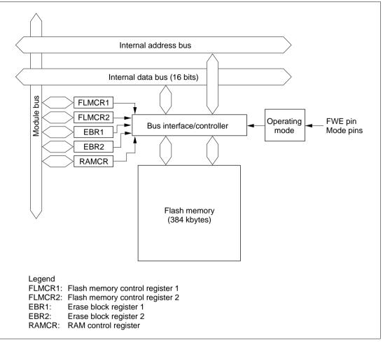
Figure 18.1 Block Diagram of Flash Memory
