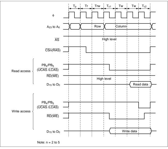
Figure 6.20 Example of Wait State Insertion Timing (CSEL = 0)
