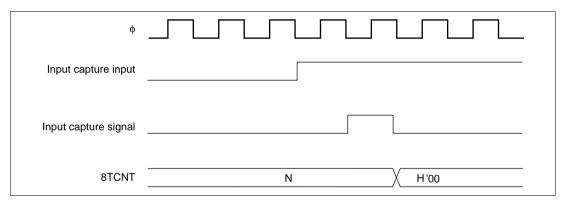
Figure 10.12 Timing of Clear by Input Capture
