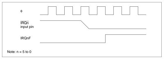
Figure 5.3 Timing of Setting of IRQnF
