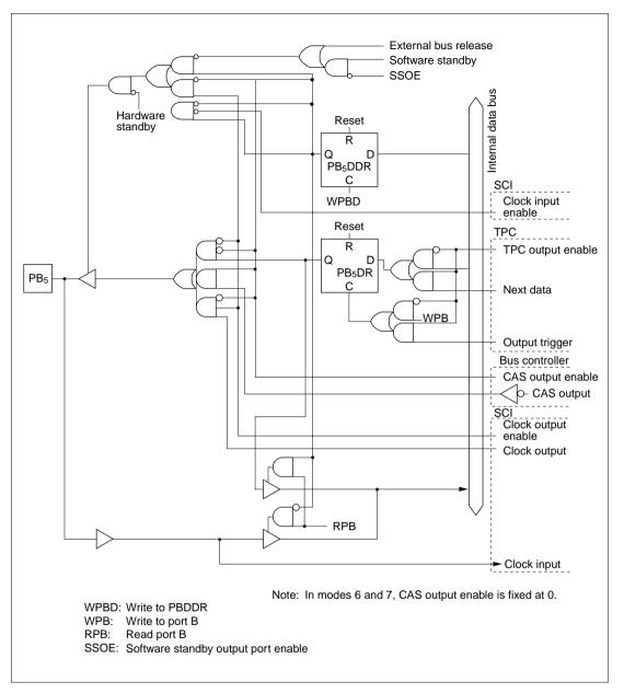
Figure C.11 (f) Port B Block Diagram (Pin PB5)
