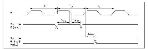
Figure 21.17 TPC and I/O Port Input/Output Timing
