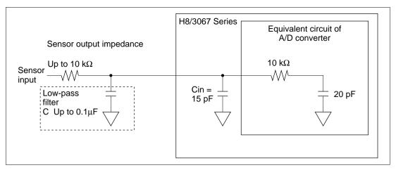
Figure 15.11 Analog Input Circuit (Example)
