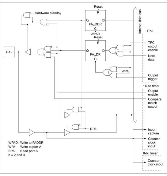
Figure C.10 (b) Port A Block Diagram (Pins PA<sub>2</sub>, PA<sub>3</sub>)
