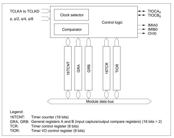
Figure 9.2 Block Diagram of Channels 0 and 1
