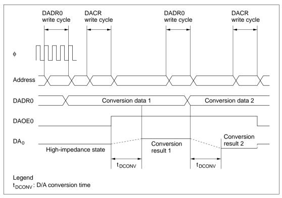
Figure 16.2 Example of D/A Converter Operation
