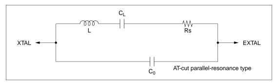
Figure 19.3 Crystal Resonator Equivalent Circuit
