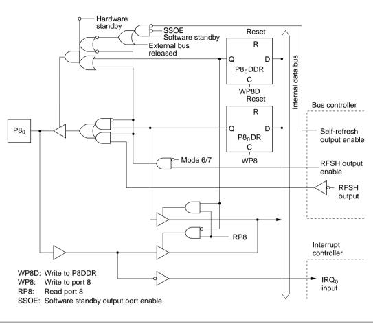
Figure C.8 (a) Port 8 Block Diagram (Pin P80)
