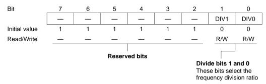
DIVCR is initialized to H'FC by a reset and in hardware standby mode. It is not initialized in software standby mode.
