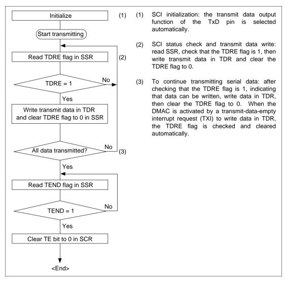
Figure 13.16 Sample Flowchart for Serial Transmitting
