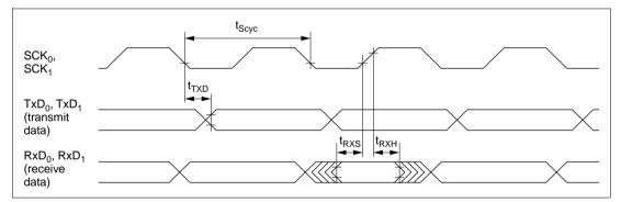
Figure 21.21 SCI Input/Output Timing in Synchronous Mode
