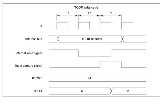
Figure 10.23 Contention between TCOR Write and Input Capture
