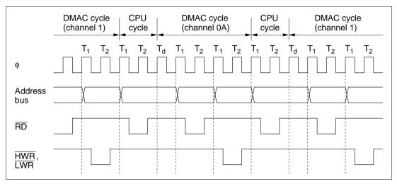
Figure 7.19 Timing of Multiple-Channel Operations
