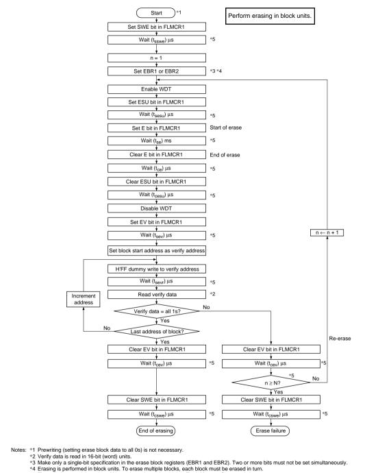
\*5 The wait times and the value of N are shown in section 21.1.6, Flash Memory Characteristics.
