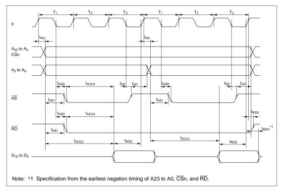
Figure 21.12 Burst ROM Access Timing: Three-State Access
