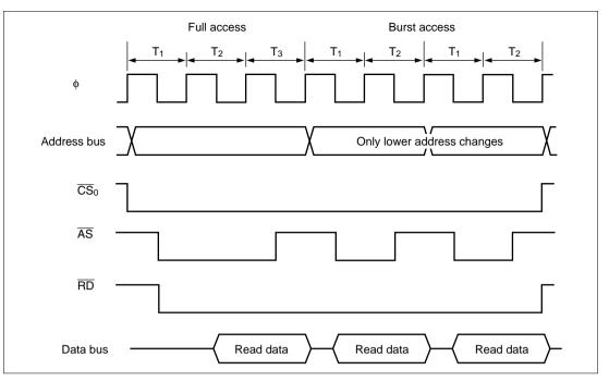
Figure 6.42 Example of Burst ROM Access Timing
