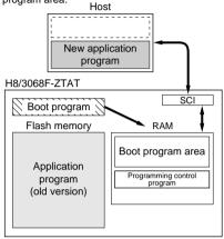
4. Writing new application program The programming control program transferred from the host to RAM is executed, and the new application program in the host is written into the flash memory.
