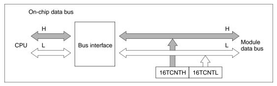
Figure 9.8 Access to Timer Counter H (CPU Reads 16TCNTH, Upper Byte)
