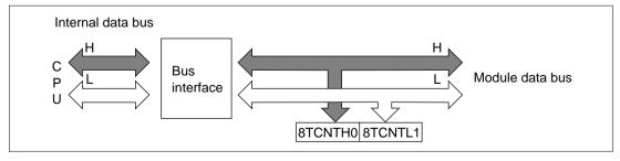
Figure 10.4 8TCNT0 Access Operation (CPU Writes to 8TCNT0, Upper Byte)
