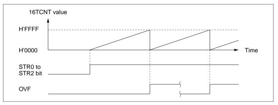
Figure 9.13 Free-Running Counter Operation
