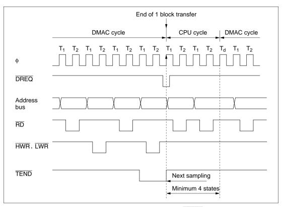
Figure 7.18 Timing of DMAC Activation by Falling Edge of DREQ in Block Transfer Mode
