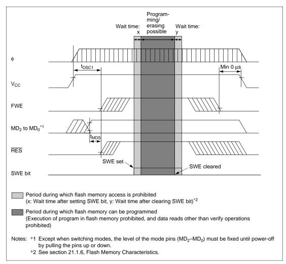
Figure 18.17 Power-On/Off Timing (User Program Mode)
