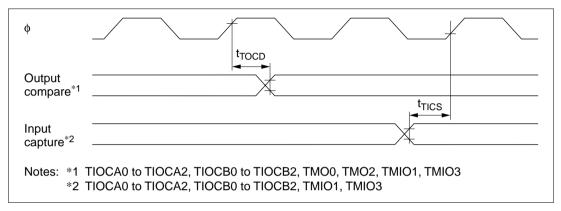
Figure 21.18 Timer Input/Output Timing
