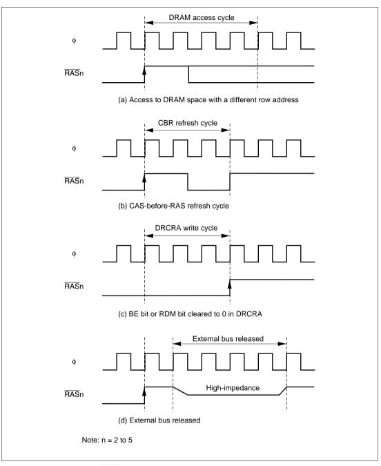
Figure 6.24 RASn Negation Timing when RAS Down Mode is Selected
