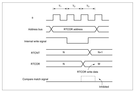
Figure 6.41 Contention between RTCOR Write and Compare Match
