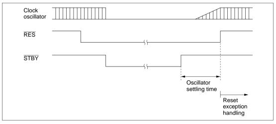
Figure 20.2 Hardware Standby Mode Timing
