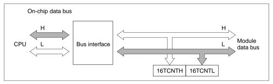
Figure 9.7 Access to Timer Counter L (CPU Writes to 16TCNTL, Lower Byte)
