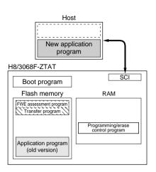
Writing new application program Next, the new application program in the host is written into the erased flash memory blocks. Do not write to unerased blocks.
