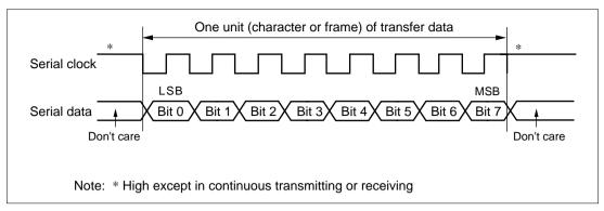
Figure 13.14 Data Format in Synchronous Communication
