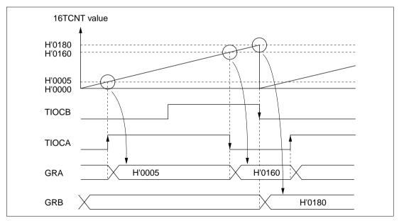
Figure 9.22 Input Capture (Example)
