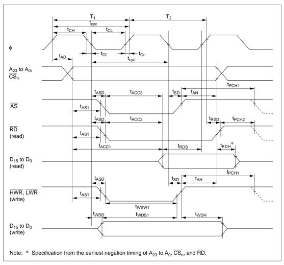
Figure 21.8 Basic Bus Cycle: Two-State Access
