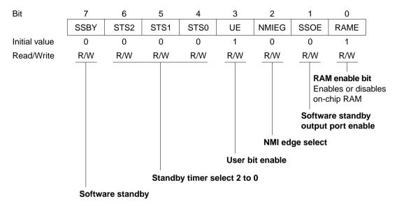
One function of SYSCR is to enable or disable access to the on-chip RAM. The on-chip RAM is enabled or disabled by the RAME bit in SYSCR. For details about the other bits, see section 3.3, System Control Register (SYSCR).
