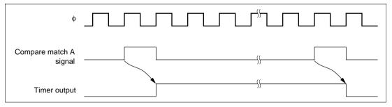
Figure 10.10 Timing of Timer Output
