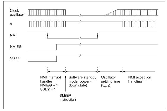
Figure 20.1 NMI Timing for Software Standby Mode (Example)
