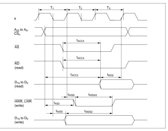
Figure 21.9 Basic Bus Cycle: Three-State Access
