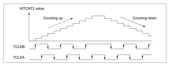
Figure 9.30 Operation in Phase Counting Mode (Example)
