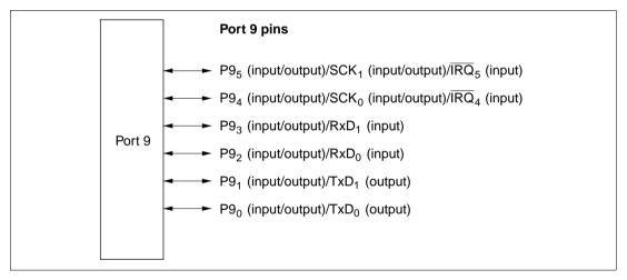
Figure 8.9 Port 9 Pin Configuration
