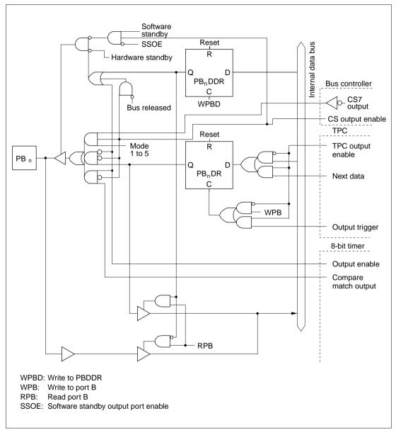
Figure C.11 (a) Port B Block Diagram (Pin PB<sub>0</sub>)
