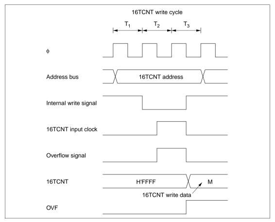
Figure 9.41 Contention between 16TCNT Write and Overflow
