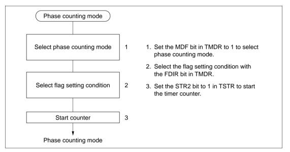
Figure 9.29 Setup Procedure for Phase Counting Mode (Example)
