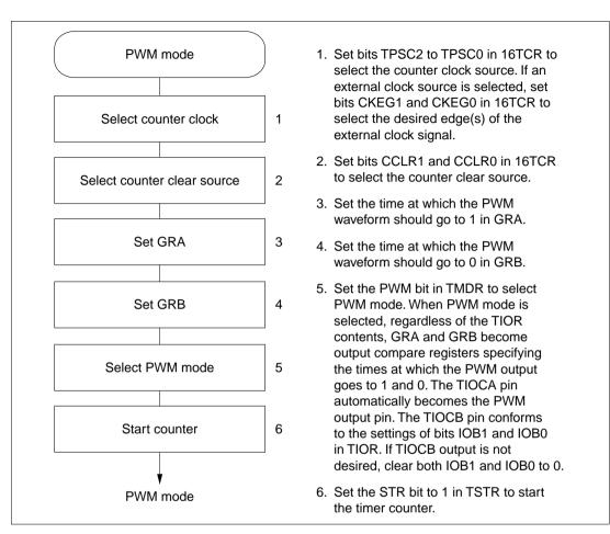
Figure 9.26 Setup Procedure for PWM Mode (Example)
