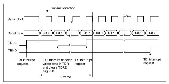
Figure 13.17 shows an example of SCI transmit operation.
