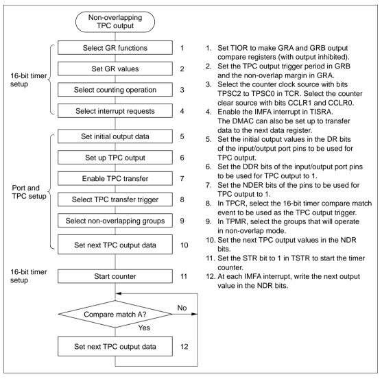
Figure 11.6 Setup Procedure for Non-Overlapping TPC Output (Example)
