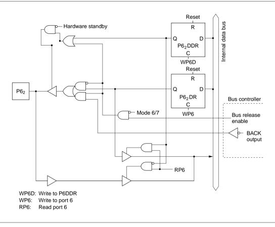
Figure C.6 (c) Port 6 Block Diagram (Pin P6<sub>2</sub>)
