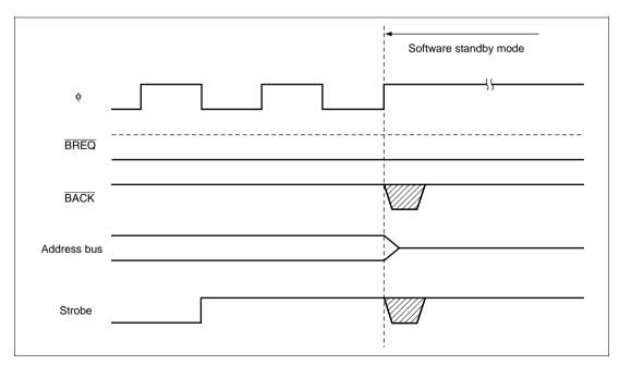
Figure 6.36 Bus-Released State and Software Standby Mode
