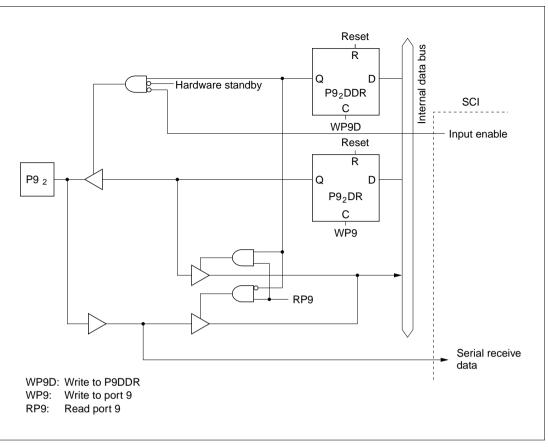
Figure C.9 (c) Port 9 Block Diagram (Pin P9<sub>2</sub>)
