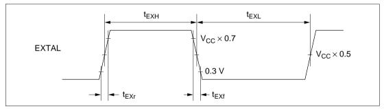
Figure 19.6 External Clock Input Timing
