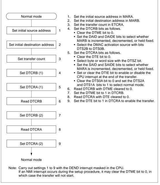
Figure 7.9 Normal Mode Setup Procedure (Example)
