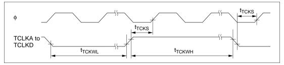
Figure 21.19 Timer External Clock Input Timing
