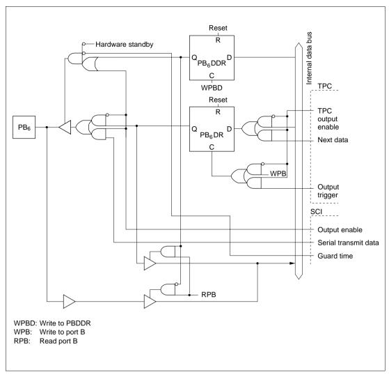
Figure C.11 (g) Port B Block Diagram (Pin PB<sub>6</sub>)
