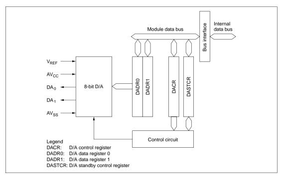
Figure 16.1 D/A Converter Block Diagram
