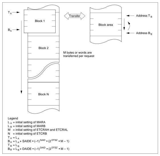
Figure 7.10 Operation in Block Transfer Mode
